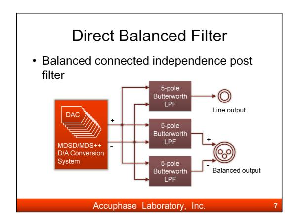
Full-balanced structure is employed after D/A converter in DC-37.
